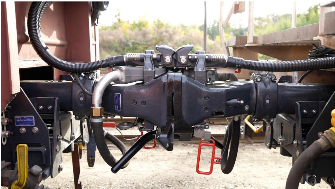
Figure 1: Photo of two coupled DACs by VOITH (Voith GmbH & Co. KGaA, 2022).
